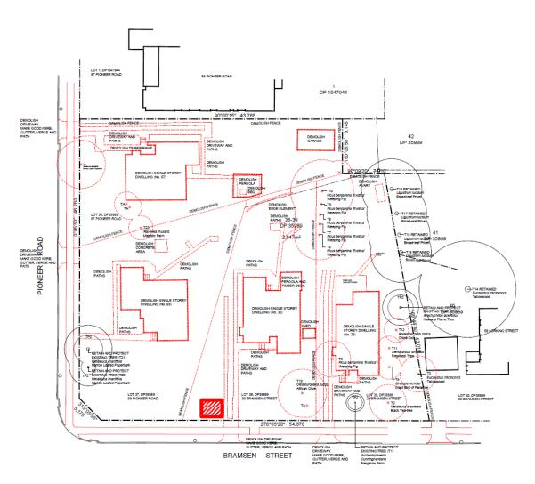
Source: Mcintosh Phelps Architecture, 67-69 Pioneer Rd and 28-30 Bramsen St Bellambi NSW, Drawing No A004 Rev D – Demolition Plan
